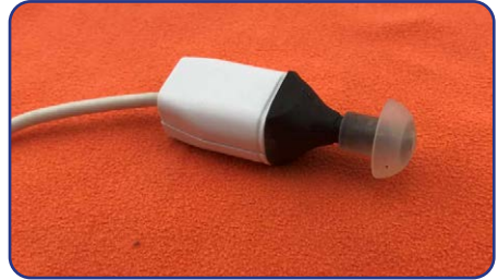
Assembled probe with injection moulded parts design
