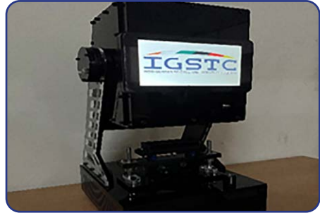
Fabricated Array Fiber-Optic Biosensor
