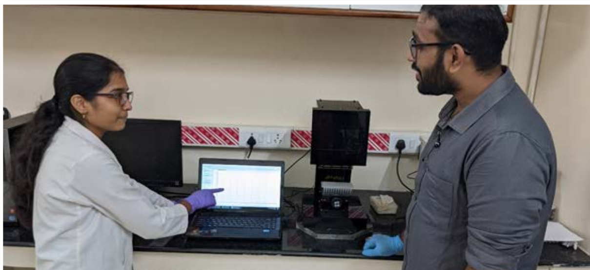
Fiberoptic Array Biosensor: A Compact array biosensor with 8 probes for simultaneous detection of up to 7 different pathogens of interest.
